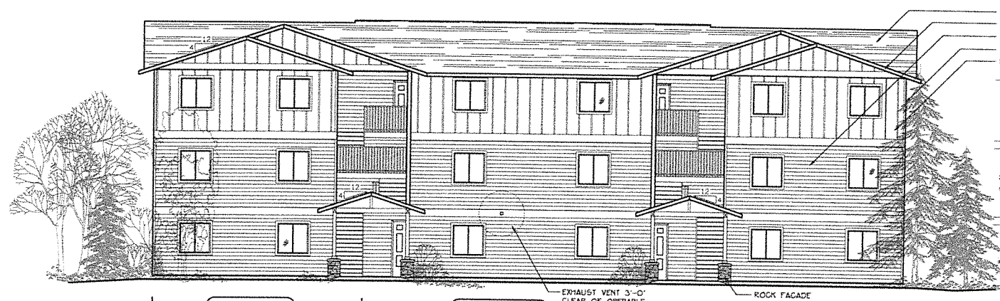
TYPE D UNIT | TYPE C UNITS | EXHAUST VENT 3'-0" CLEAR OF OPERABLE WINDOW AREA TYP. | ROCK FACADE | TYPE D UNIT | NORTH ELEVATION (BLD. 2) SCALE: 1/8" = 1'-0"
