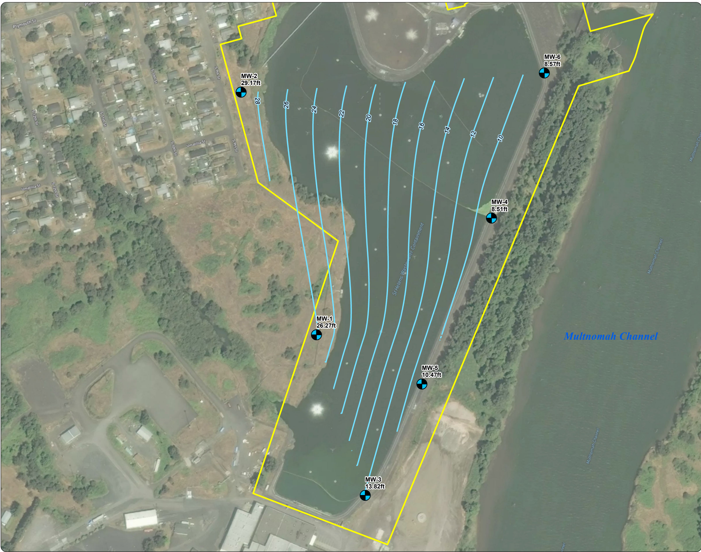
Figure 8-1 August 2019 Groundwater Elevations City of St. Helens Wastewater Treatment Lagoon St. Helens, Oregon
