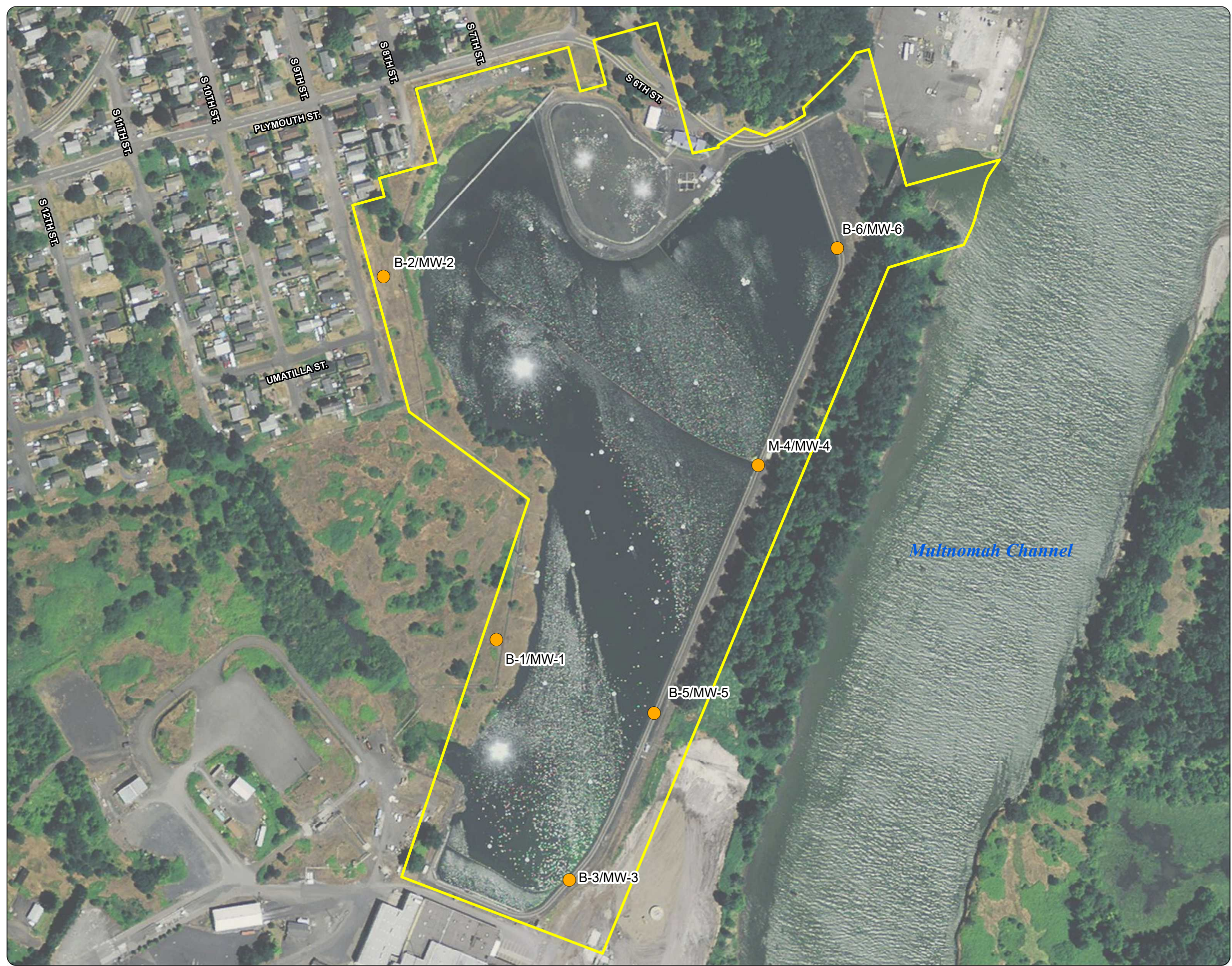
Figure 7-1 Boring and Monitoring Well Locations City of St. Helens Wastewater Treatment Lagoon St. Helens, Oregon
