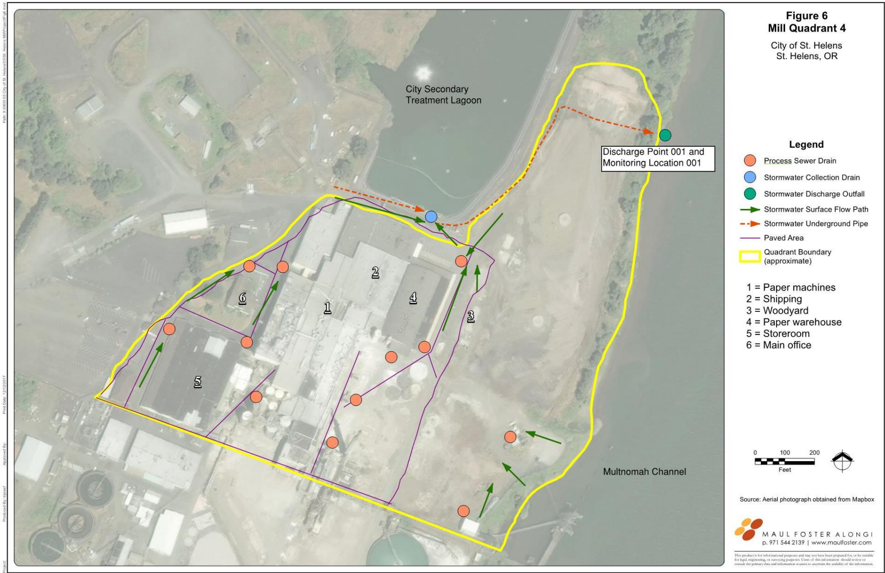
Figure 13. Quadrant 4 Utilities Map (Figure 4 from 2017 SWPCP)
