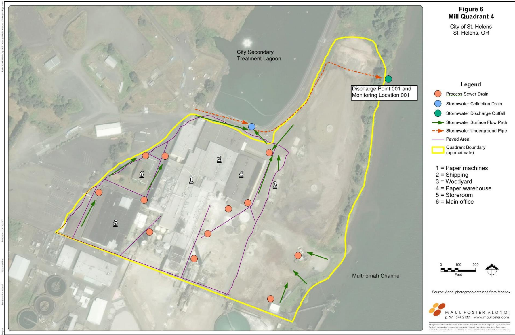
Figure 13. Quadrant 4 Utilities Map (Figure 4 from 2017 SWPCP)
