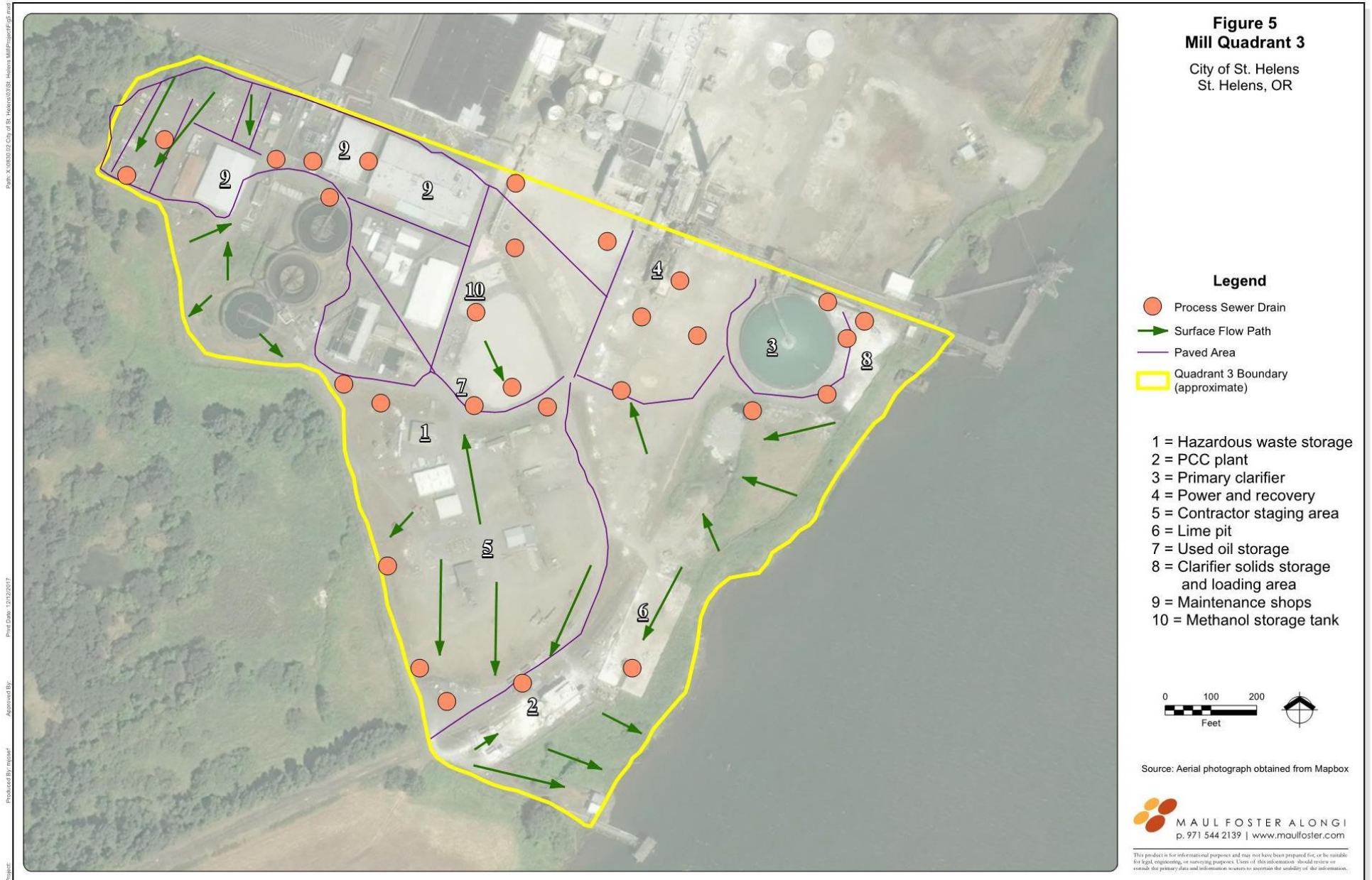
Figure 12. Quadrant 3 Utilities Map (Figure 5 from 2017 SWPCP)
