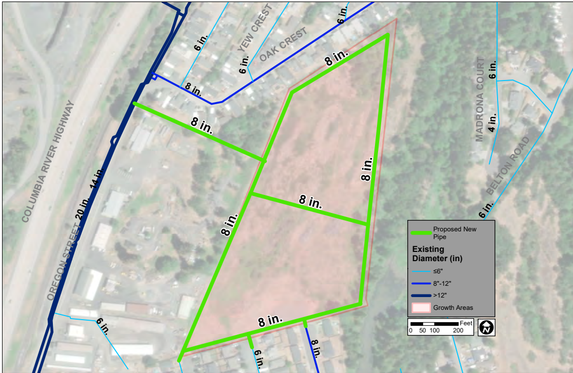
FIGURE 5-12: GROWTH AREA 12, 14, AND 15 PROPOSED PIPING
