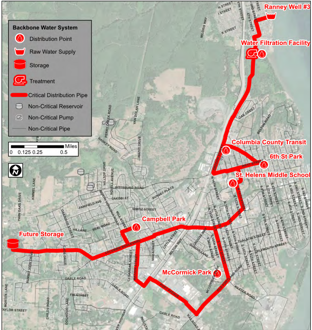
FIGURE 1-7: BACKBONE WATER SYSTEM
