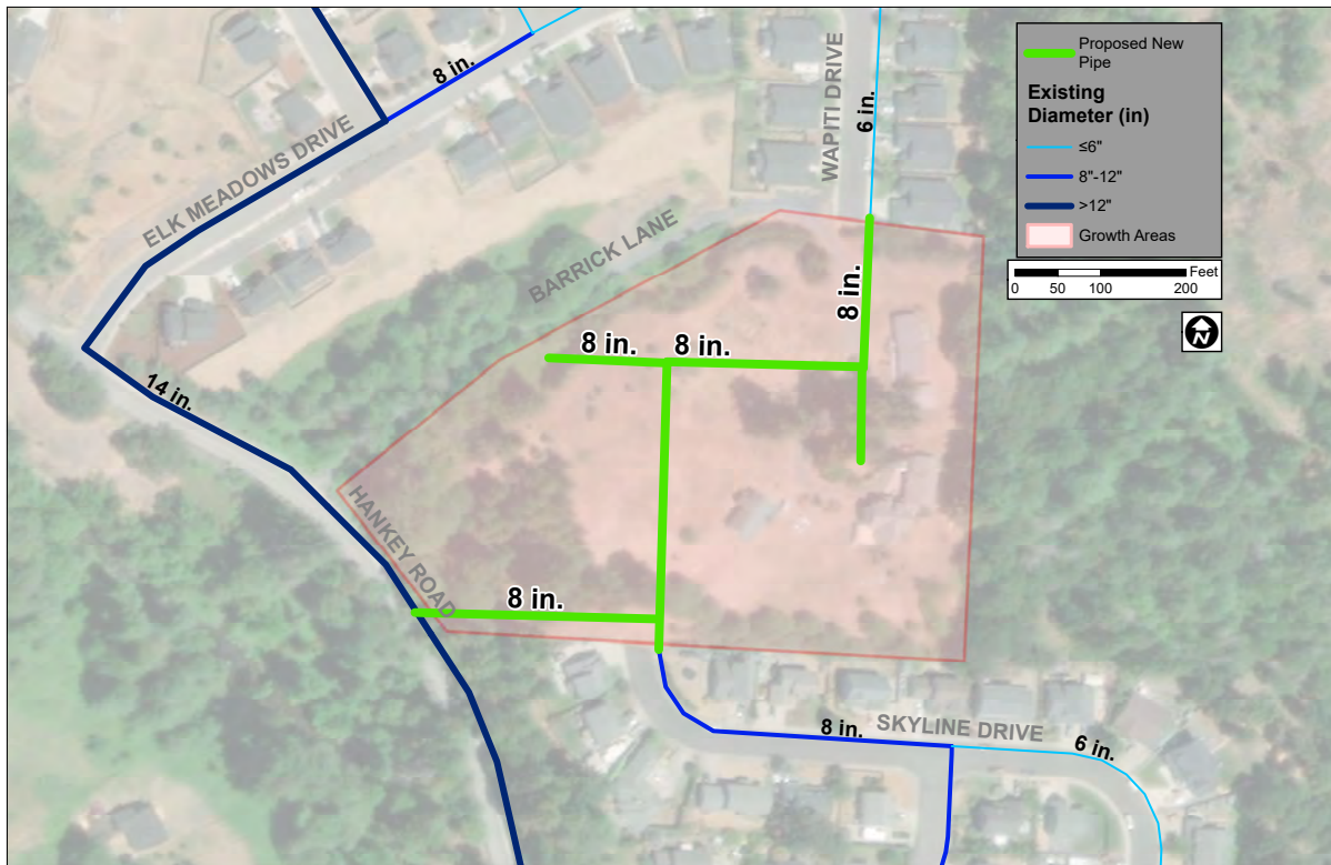
FIGURE 5-10: GROWTH AREA 6 PROPOSED PIPING
