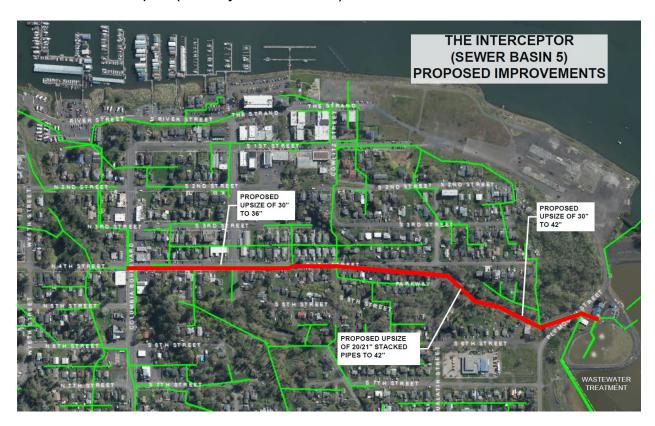
The Interceptor (also called Sewer Basin 5 or the "The Tunnel"), collects flows from four sewer basins before conveying flows to the WWTP.
