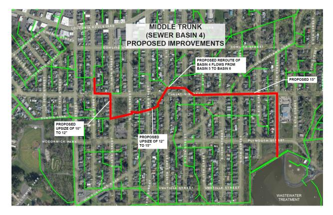
The Middle Trunk has high I/I rates, has the largest concentration of potential overflow locations, and contributes to the surcharging in the Interceptor (Basin 5). By rerouting some of the flow away from the Interceptor, Basin 5 trunkline may experience reduced surcharging. It is recommended in the WWMP that improvements to the Middle Trunk be constructed prior to the upsizing the Basin 5 pipeline.
