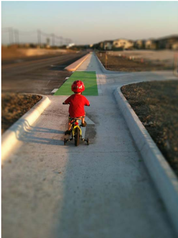
Grade-separated cycletrack with driveway in Austin, TX
