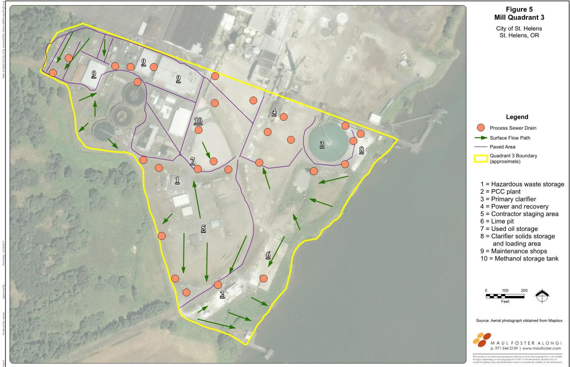
Figure 12. Quadrant 3 Utilities Map (Figure 5 from 2017 SWPCP)
