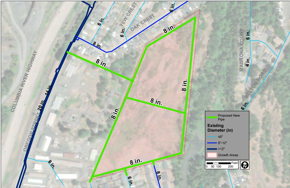
FIGURE 5-12: GROWTH AREA 12, 14, AND 15 PROPOSED PIPING
