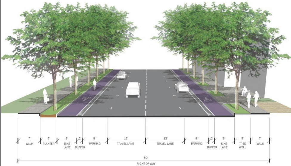
S 1ST STREET CROSS-SECTION - BUFFERED BIKE LANES
